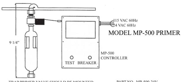
TRAP PRIMER VALVE SHOULD BE MOUNTED ONE FOOT ABOVE THE FINISHED FLOOR FOR EVERY 20 FEET OF PRIMER LINE.
